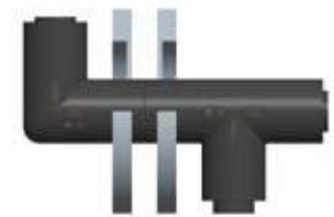
6. Weld the pipes and let them cool off
