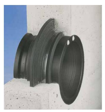
The concrete connection socket is mounted flush with the formwork and grouted in with concrete. A prefabricated groove guarantees safe anchoring and the puddle flange acts as a seal.
